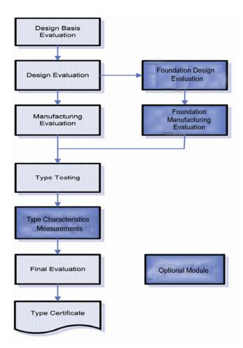
Figure 10. Type certification procedure according to IEC 61400-22.
