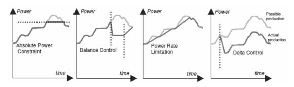
Figure 6. Potential wind farm control mechanisms to regulate grid loading<sup>15</sup>.
